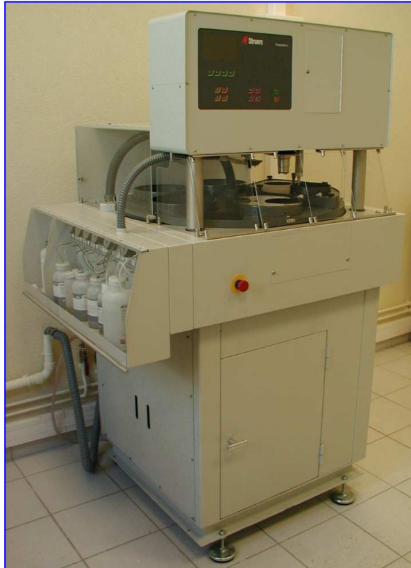
Figure 132 – Robot de polissage (Struers PREPAMATIC).
