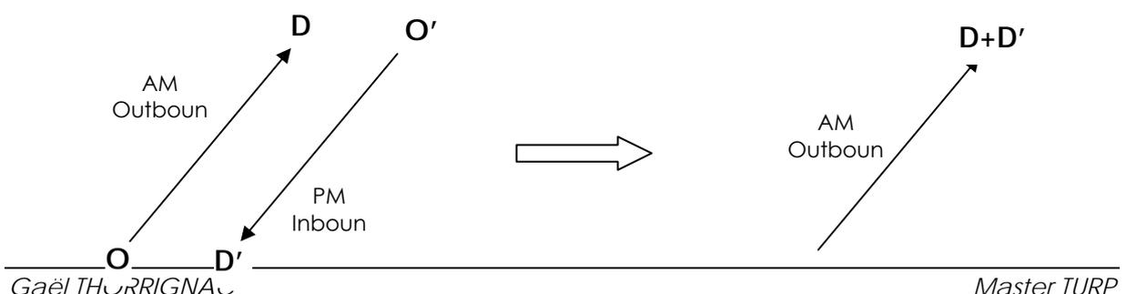
In that way, all information from the Raw RSI data can be collected in only one OD distribution for the AM period. It is to point out the building of these data took in the surveyed counts for all the survey period (7:00 - 11:00 and 15:00 - 19:00): this procedure was necessary as the number of trips counted in the desired AM peak period (8:00 - 9:00) was considered insufficient to make a consistent trips estimation.
