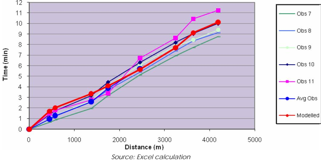
**Figure 28: Comparison of modelled and observed travel times across the corridor (AM period, south bound)**
