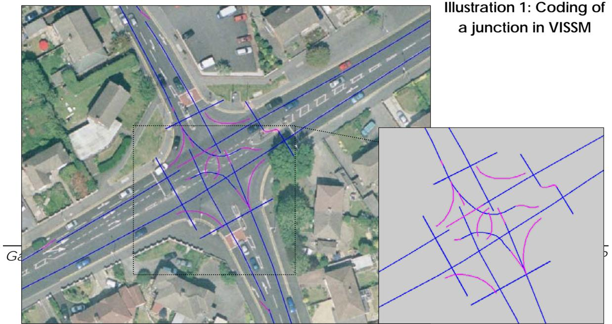
**Illustration 1: Coding of a junction in VISSIM**
