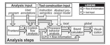
Figure 1.3: Core components of a timing-analysis tool
