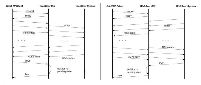
Figure 13: Data interaction for the BlobSeer Asynchronous Approach: put (left), get (right)
