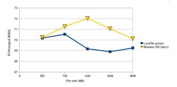
Figure 15: I/O througput performance when large data files transferred
