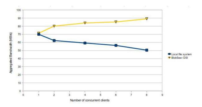
Figure 16: Aggregated througput of local file DSI and BlobSeer DSI asynchronous approach when concurrent clients put different files into storage
