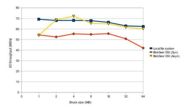
Figure 14: I/O access comparison between local file system DSI, BlobSeer DSI synchronous and aysnchronous approaches
