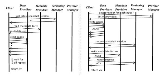
Figure 8: Internal interactions inside BlobSeer: READ(left) and WRITE(right).
