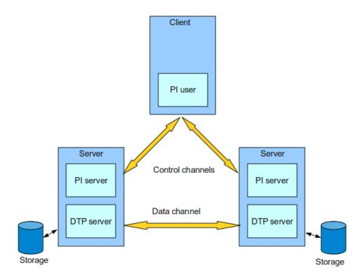
Figure 5: The striped GridFTP configuration
