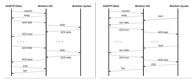
Figure 12: Data interaction for the BlobSeer Synchronous Approach: put (left), get (right)
