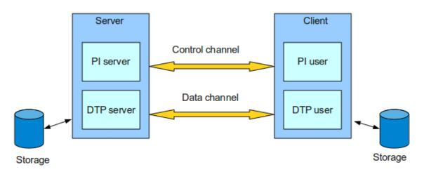
Figure 4: The non-striped GridFTP configuration
