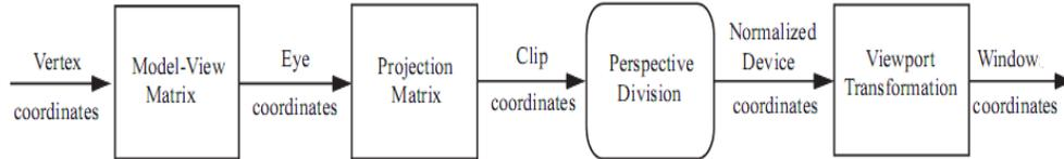
FIGURE 4.3.1: Pipeline OpenGL
