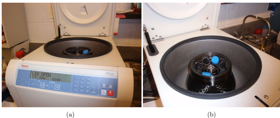
Figure 31: Centrifuge Sorvall LEGEND X1 : filtration of the solutions to highlight the solvent effect in the CNTs dispersion
