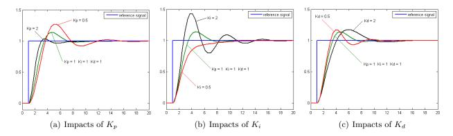
Figure 6: The impact of the gains  $(K_p, K_i \text{ and } K_d)$  on the output value [1]
