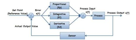
Figure 5: PID controller, general diagram
