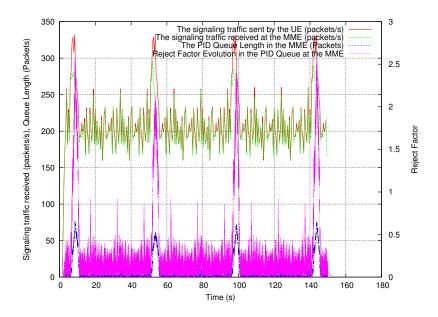
Figure 21: The Reject Factor evolution depending on the signaling traffic received and the queue length in the MME in case of Uniform traffic with bursts
