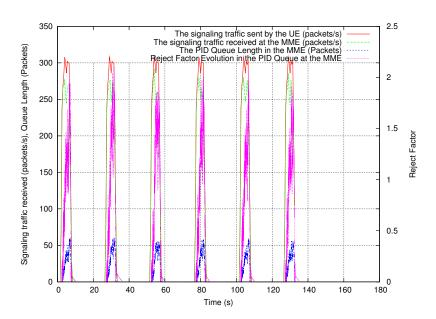
Figure 13: The Reject Factor evolution depending on the signaling traffic received and the queue length in the MME in case of Bursty traffic
