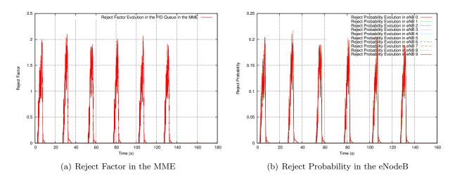
Figure 12: The Reject Factor evolution in the MME and the Reject Probabilities in the different eNodeBs in case of Bursty traffic
