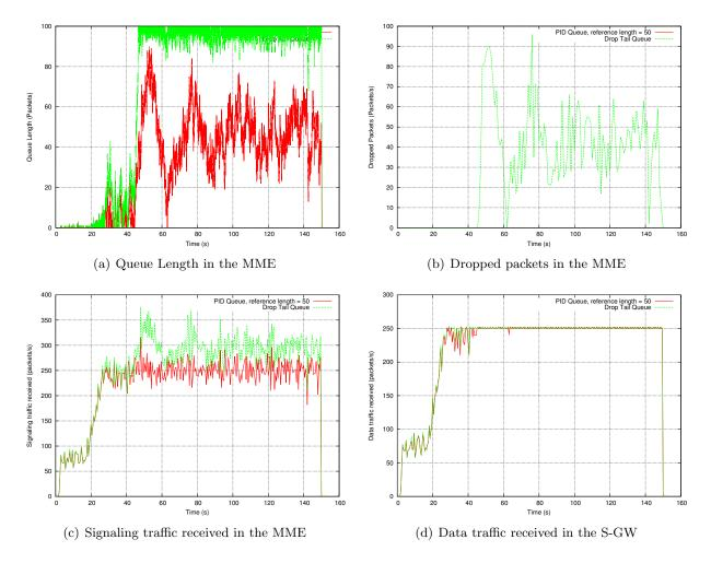
Figure 26: Comparison between the case where a PID queue and drop tail queue are used in the MME in case of Random traffic
