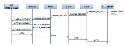
Figure 4: Sequence Diagram for signaling and data in case of Query Driven applications
