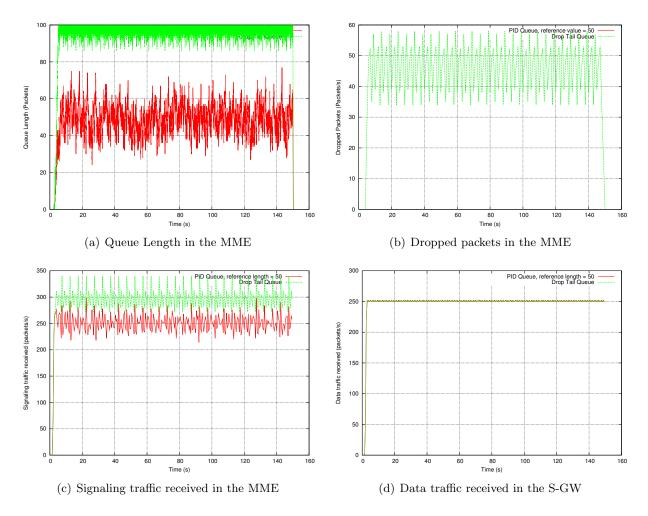
Figure 18: Comparison between the case where a PID queue and drop tail queue are used in the MME in case of Uniform traffic
