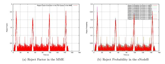
Figure 20: The Reject Factor evolution in the MME and the Reject Probabilities in the different eNodeBs in case of Uniform traffic with bursts
