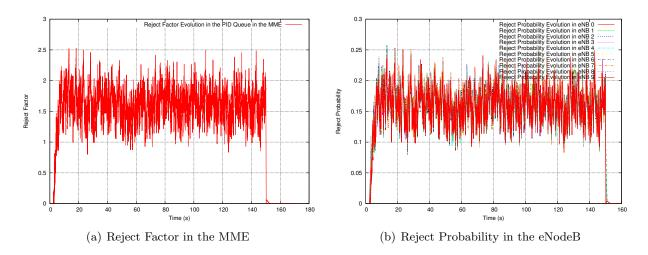
Figure 16: The Reject Factor evolution in the MME and the Reject Probabilities in the different eNodeBs in case of Bursty traffic
