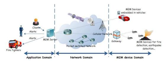
Figure 1: A general architecture of a M2M application
