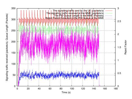
Figure 17: The Reject Factor evolution depending on the signaling traffic received and the queue length in the MME in case of Uniform traffic
