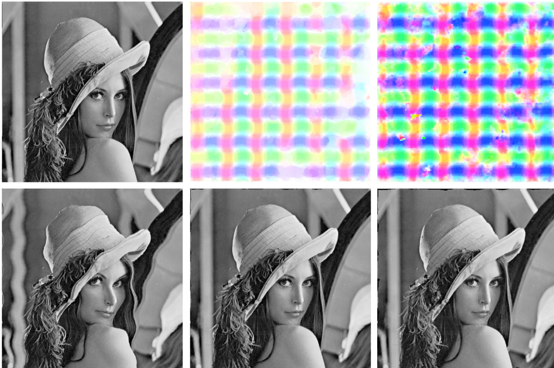
Figure A.9: Result of the 2D optical flow on lena.pgm and lena.pgm transformed by a 2D sine wave.
