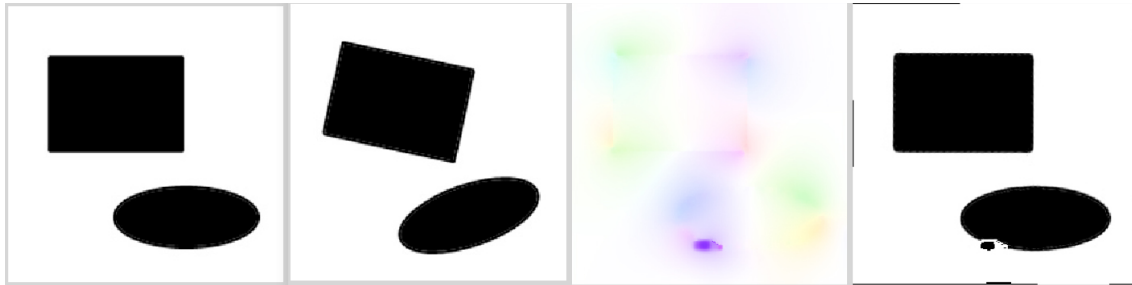
Figure A.8: 2D optical flow algorithm in matlab. From left to right: 1. two black shapes, 2. the same black shapes rotated, 3. the resulting flow field, and 4. the restored shapes.
