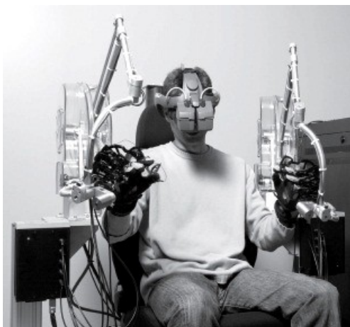
Figure 2.1: Bi-manual Haptic-workstation system (from [Ott09])
