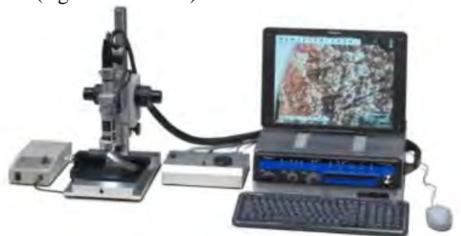
Fig. 14. Microscope HIROX KH-7700, C2RMF http://www.hirox-europe.com/
