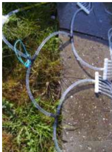
Figure 3: 2x2x6 mouthpieces division to supply the 24 grazing chambers
