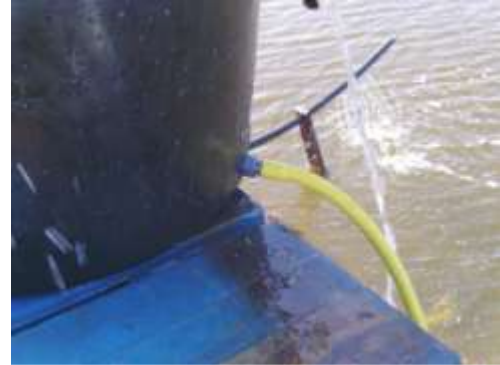
Figure 2: Main water supply to the system, after the height levelled bucket
