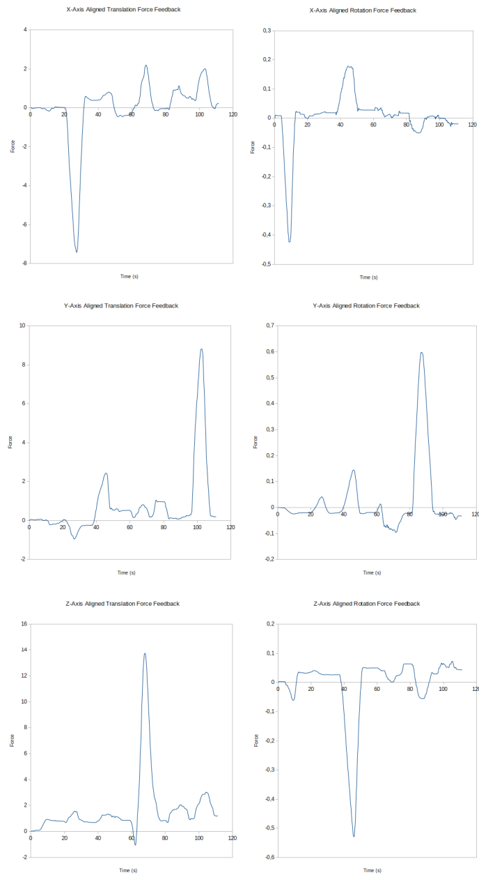
Figure 6.7: Force feedback for each dimension, both in translation and in rotation. For 0 \leq t \leq 20 we have a rotation around the x-axis, followed by a translation along the x-axis for 20 \leq t \leq 40 . Then for 40 \leq t \leq 60 we have a translation along the z-axis, followed by a rotation around the z-axis for 60 \leq t \leq 80 . We finally have for 80 \leq t \leq 100 we have a rotation around the y-axis, followed by a translation along the y-axis for 100 \leq t \leq 120 .
