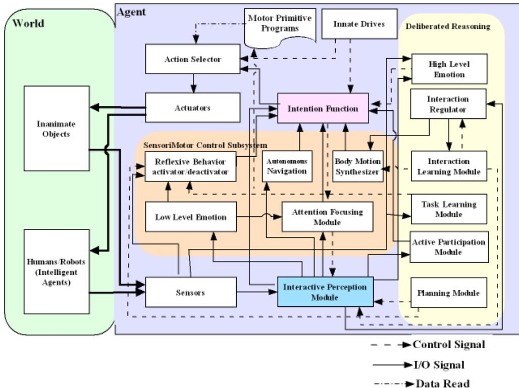
FIGURE 5 – Embodied Interactive Control Architecture (EICA).
