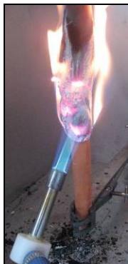
Figure 5.7 : Application de la flamme
