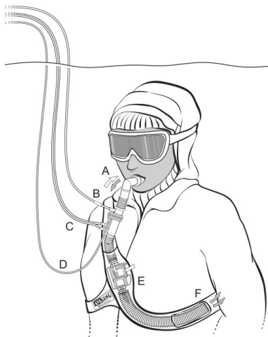
Fig. 2. Breathing device used during the hypercapnic study burial (Avalung 2, Black Diamond Equipment, Salt Lake City, UT). Open arrow shows flow of inspiratory air, and shaded arrows show flow of expiratory air. The subject breathes in and out through the mouthpiece (A). An emergency oxygen backup line (B) is attached directly into the mouthpiece apparatus and is used only if the subject becomes hypoxic or requests to end the study. Monitoring lines (C and D) are connected to a capnometer and record inspiratory PCO_2 , end-tidal PCO_2 , and minute ventilation (VE). Inhaled air enters from the snowpack through the 1-way inspiratory valve on the side of the housing inside the mesh-protected harness on the chest (E). Expired air leaves the lungs through the mouthpiece and travels down the respiratory tubing to the housing and then passes through an expiratory 1-way valve located at the bottom of the housing (E) and travels via respiratory tubing inside the harness around to the back (F).
