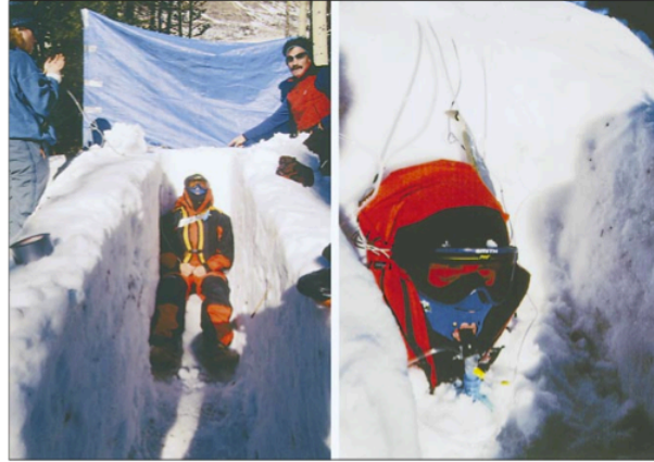
The left panel shows the compacted snow mound with a subject sitting in the trench in burial position. The right panel shows the subject buried to the neck prior to full burial. The device mouthpiece with capnometer tubing, emergency oxygen tubing, and physiologic monitoring cables is visible.
