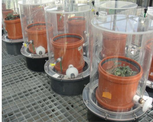
Figure 6. Microcosms in transparent containers during <sup>13</sup>CO<sub>2</sub> labelling. 10 ml of <sup>13</sup>CO<sub>2</sub> was inserted into a valve on the container wall with a gastight syringe. Agroscope, AL. Corbel, 2014.
