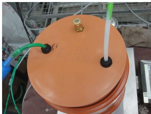
Figure 3 with a removable cap with two valves for N<sub>2</sub>O samples. Agroscope, AL. Corbel, 2014.
