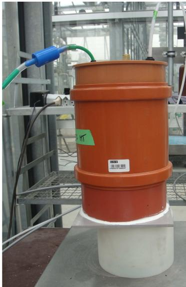
Figure 4 Enclosed microcosm during a N<sub>2</sub>O gas measurement. Agroscope, AL. Corbel, 2014.
