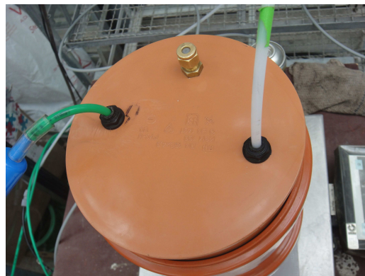
Figure 3 with a removable cap with two valves for N 2 O samples. Agroscope, AL. Corbel, 2014.
