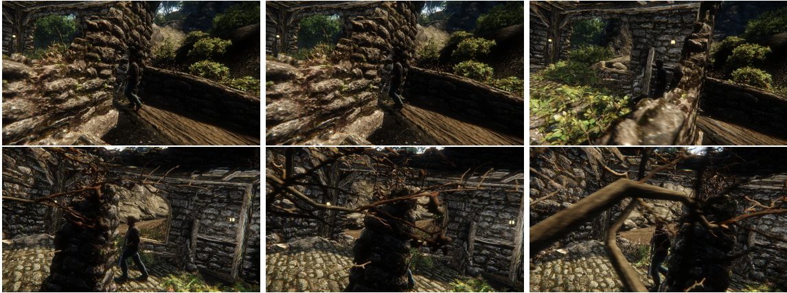
Figure 20: In both these sequences we can see the actor before, during and after occlusion. Here our threshold is set to 0.6 seconds. This means that if the actor is to be invisible for 0.6 seconds or more we change the trajectory. For the two frames we can see that the trajectory does not change for little occlusions since they last respectively 0.3 and 0.4 seconds.
