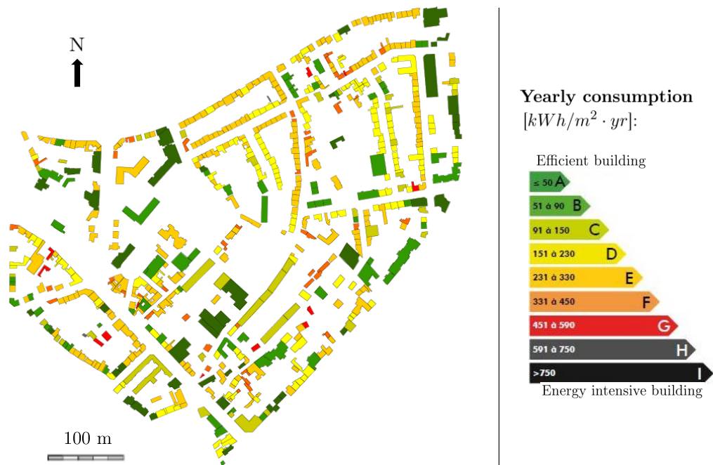
Figure 3.2: Displaying of the yearly energy consumption for heatings of St Félix buildings. Green buildings are more efficient than red ones
