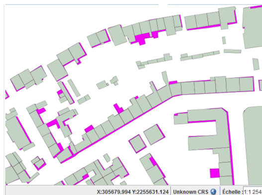
Figure 2.1: Displaying of mismatch between plot map (in grey) and topographic map (in pink)
