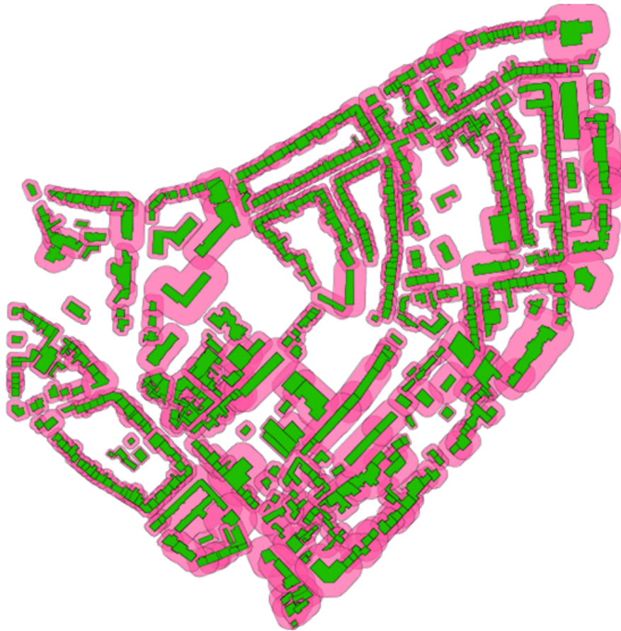
Figure 2.10: Visualization of virtual shadows (pink) around each building (green), useful for the estimation of the building obstruction impacts
