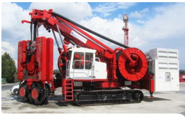
Figure 11: hydrofraise (site internet de SOLETANCHE-BACHY)
