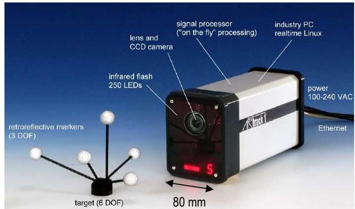
Figure 37 : ARTtrack1 de Advanced Realtime tracking GmbH, [www.ar-tracking.com](http://www.ar-tracking.com) (2006)
