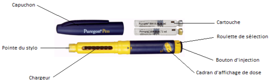
Figure 16 : Composition du stylo rechargeable PUREGON PEN®
