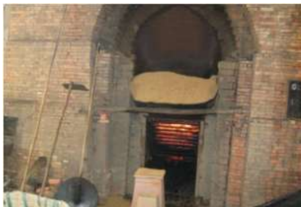
Figure 6. Rice husk burning in a kiln in Thuan Thoi village (Photo by Arvo Leinonen) (Leinonen and Nguyen 2013)
