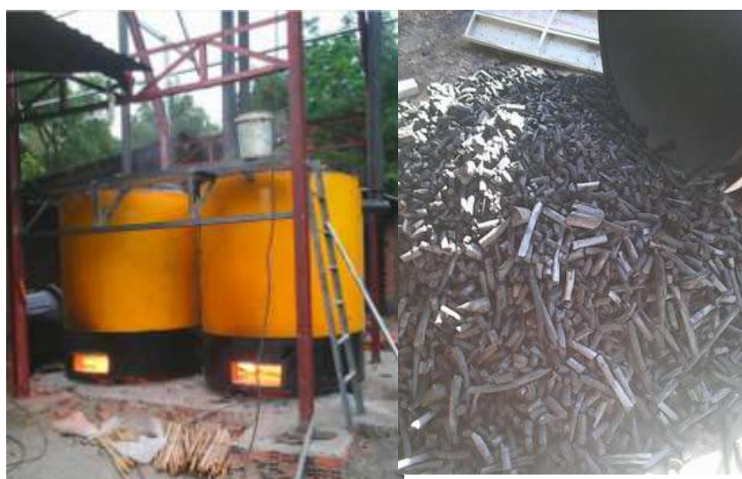
Figure 5. Pyrolysis equipment for household scale in Binh Duong (left) and charcoal product (right) (Biomass Energy Team 2014)
