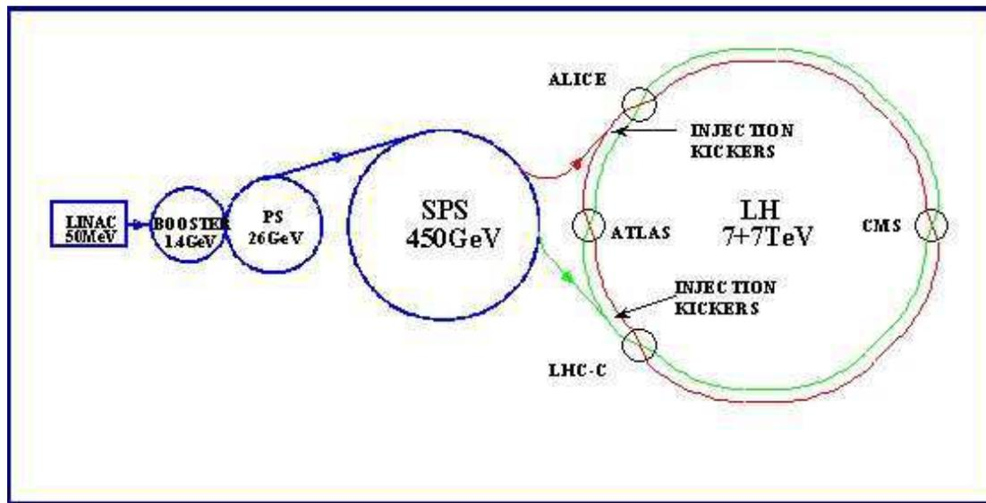
FIGURE 2.1: Layout of the acceleration chain at CERN
