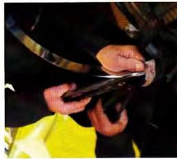
1. Cutting the Pattern - Cut lengths of tin 1 1/4" (inch) or 3cm wide by 5" or 14cm long. (This size makes a whistle suitable for a large hand). From this length cut away a length of about 1 1/2" or 4cm piece.
