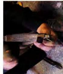
4. Shaping the Whistle End - You now need to work on the remaining section and curve it using the end of the stake and a 'scutcher'.
