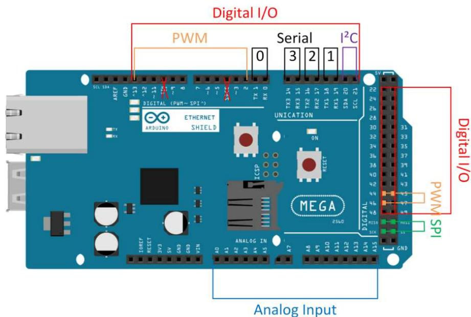
Figure 31 - Interfaces Arduino Mega et shield Ethernet
