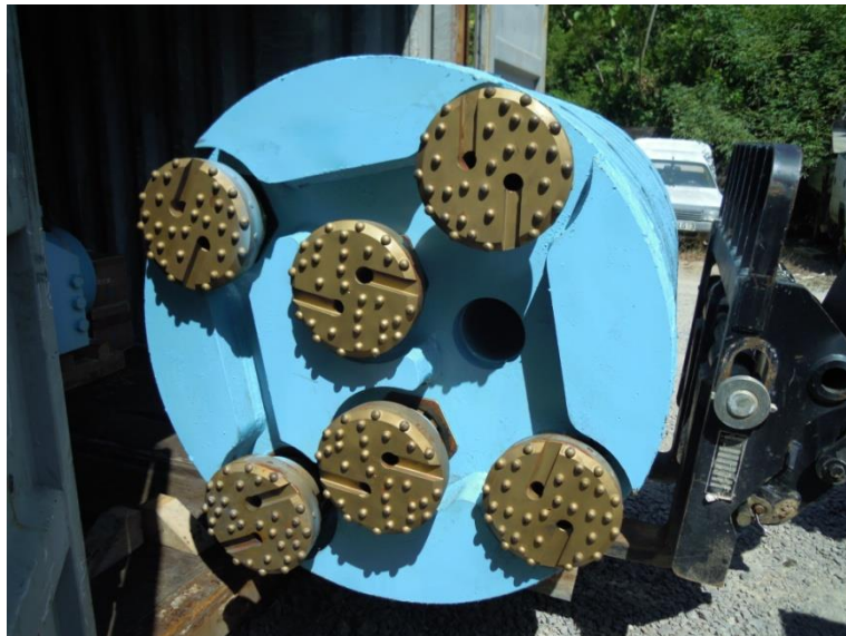
Figure 6 - Photo du barillet du cluster-drill.
