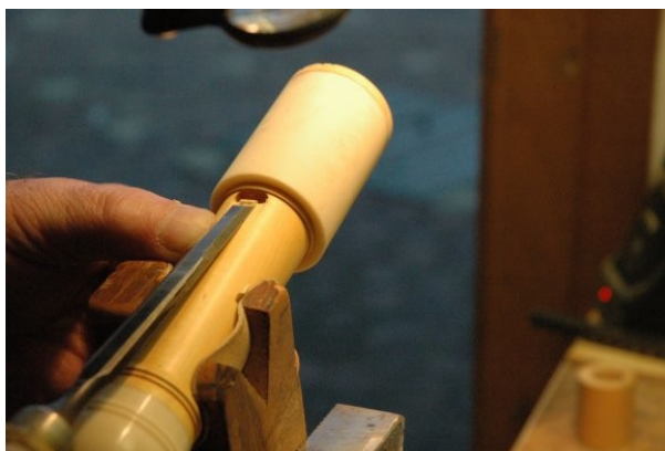
Figure 25 - Fabrication du labium - © Etienne Holmblat
