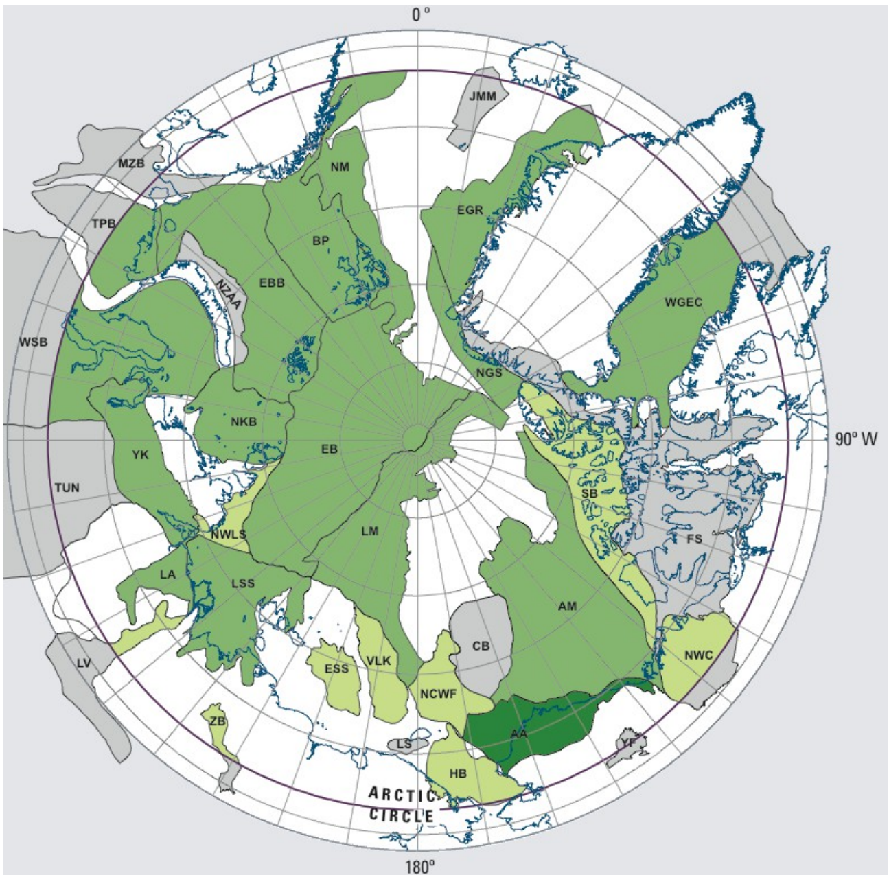
▲ Figure 3. Provinces in the Circum-Arctic Resource Appraisal (CARA) color-coded for mean estimated undiscovered oil in oil fields. Only areas north of the Arctic Circle are included in the estimates. Province labels are the same as in table 1.
