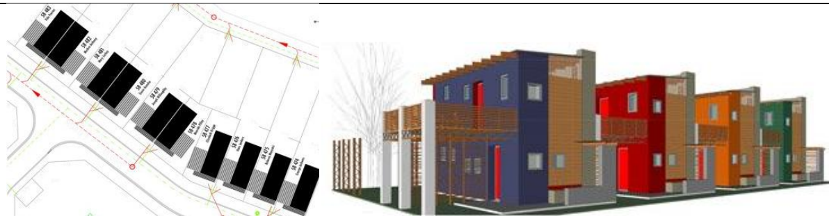
Figure 96 (Left & right) The plan and 3D perspective of the Mitchell's Plain sandbag housing project. Source: (DeZeen, 2008)
