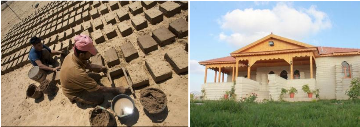
Figure 2 (Left) Production of mud bricks in Gaza. Source: (BBC News, 2009)
