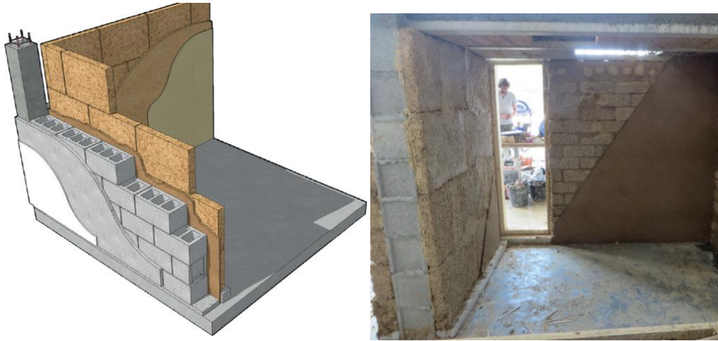
Figure 116 (Left & right) Envelope technique using light earth blocks for existing masonry structure. Source: (CRAterre, 2016)
