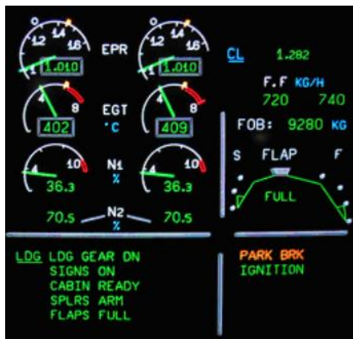
Figure 2: Example of an ECAM display (picture from skybrary.aero)
