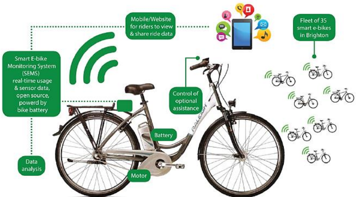
Figure 7 : The smart e-bike monitoring system (SEMS) (Source : Behrendt 2016)
