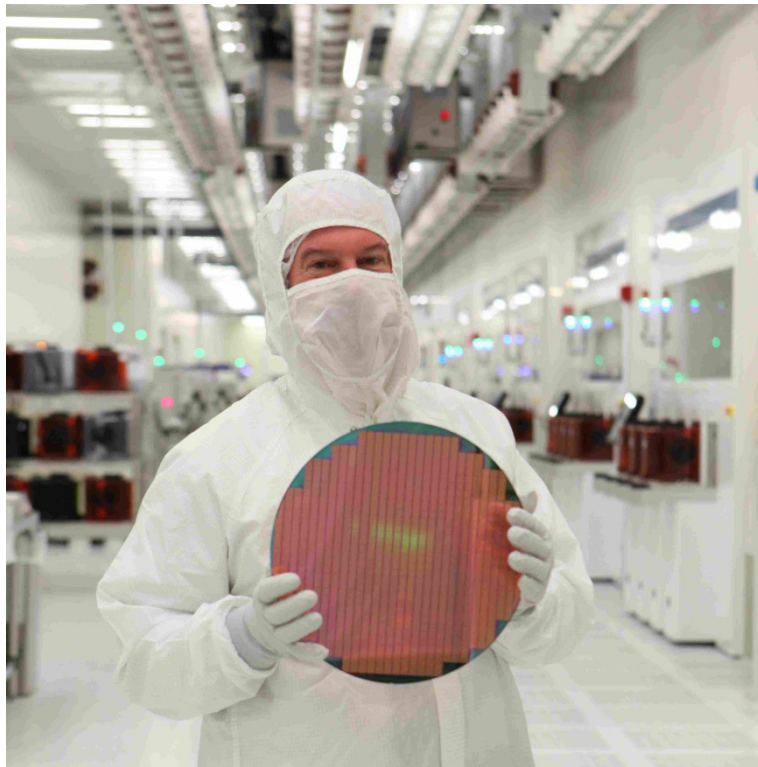
Figure 4: Picture of an engineer holding a 12 inch (30 cm) diameter wafer. He is wearing an integral suit to prevent spreading potential sources of particles
