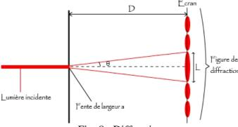
Fig. 8: Diffraction
