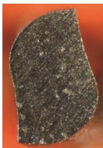
**Figure 8 : Section transversale du Reciproc (34)**
