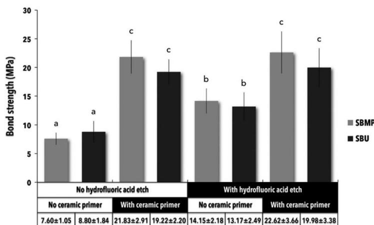
Figure 2. Mean microshear bond strengths and standard deviations of all specimen groups (MPa,  $n = 10$ ). Same letters indicate no statistically-significant difference ( $P > 0.05$ ). SBU, Scotchbond Universal Adhesive; SBMP, Adper Scotchbond Multi-Purpose Adhesive.
