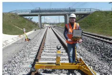
Figure 1 Chariot GRP + station totale (source C Bury)
