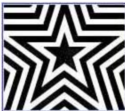
Figure 15: Test de Bowie-Dick conforme
