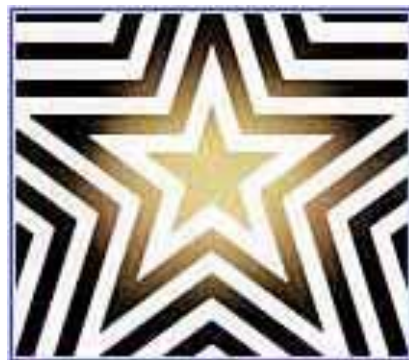
Figure 14: Test de Bowie-Dick non conforme
