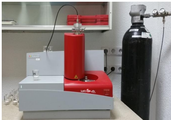
Figure 28 – Thermogravimetric and differential thermal analysis device
