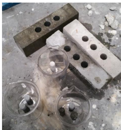
Figure 20 – Cylindrical samples for porosimetry and DTA
