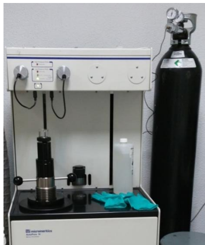
Figure 27 – Mercury Intrusion Porosimetry device
