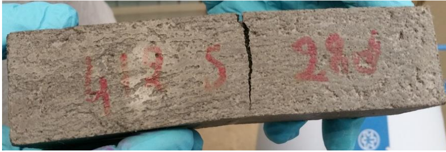
Figure 31 – Failure of a repair mortar during the tensile test
