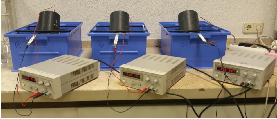
Figure 29 – Chloride migration device
