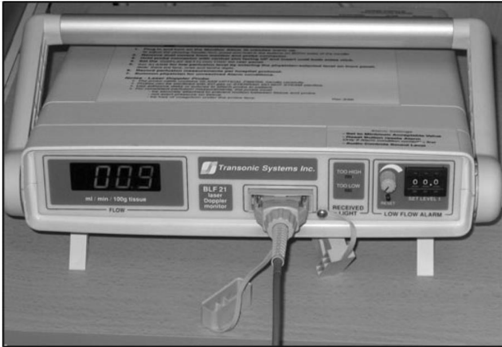
Source : Karayilmaz et Kirzioğlu, « Comparison of the reliability of laser Doppler flowmetry, pulse oximetry and electric pulp tester in assessing the pulp vitality of human teeth », 2010
