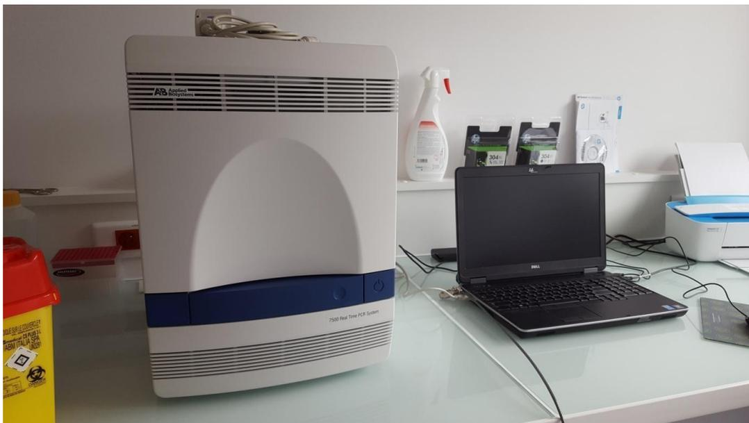
Figure 12 : Thermocycleur AB7500 (Applied Biosystems®)
