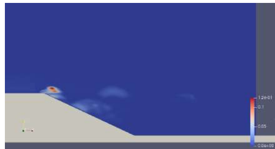
Figure 3.145: \text{nut} values over 0.1\text{m}^2/\text{s} at the rear - DES 3D kwSST simulations Mesh 3 - controlled case f/DC=180\text{Hz}/50 .
