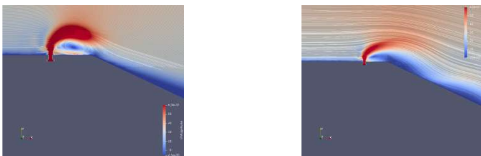
Figure 3.146: Velocity streamline - Formation of a structure of negative circulation with a strong weak pressure zone (Left) - Tilting of the structure on the ramp after a certain blowing time (right) - controlled case f/DC=180\text{Hz}/50 .
