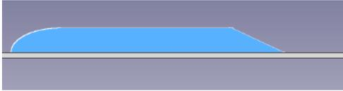
Figure 1.3: Ahmed profile for notchback vehicle - Longitudinal view
