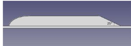
Figure 2.3: Geometrical parameters of the model - Side view
