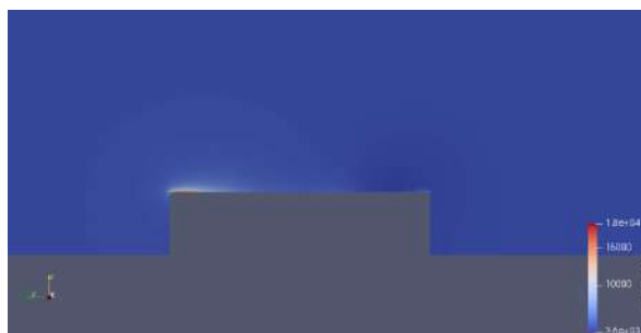
Figure 3.132: Pressure fluctuations magnitude middle plane x=1.42 - DES 3D kwSST simulations Mesh 2 - uncontrolled case.
