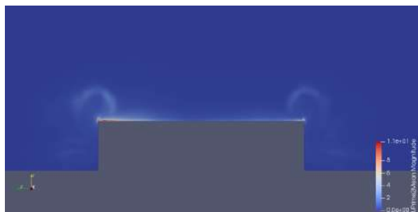
Figure 3.131: Reynolds stress magnitude plane x=1.42 - DES 3D kwSST simulations Mesh 2 - uncontrolled case.
