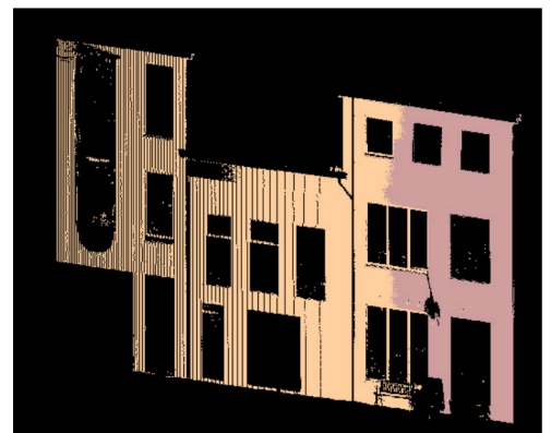
Illustration 8: Exemple de sur-segmentation (Boulaassal, 2010)
